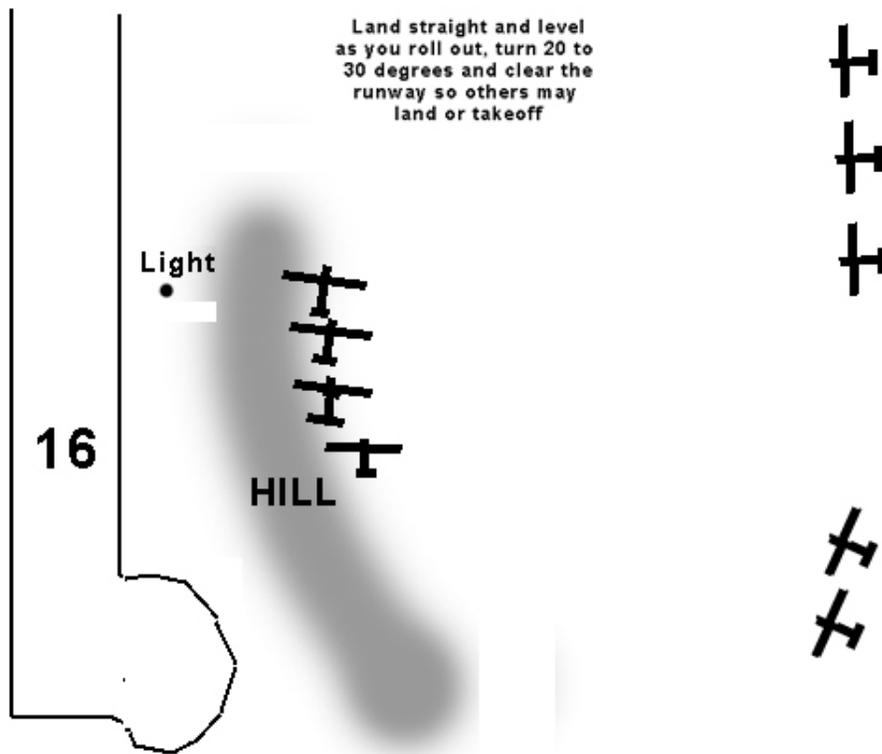
Care must be taken in moving and parking gliders in these areas. Park the gliders such that there is no possibility of collision due to sloppy movement or the wind moving them. Position the aircraft with the downwind wing on the ground, dive brakes deployed, and the canopy closed.
