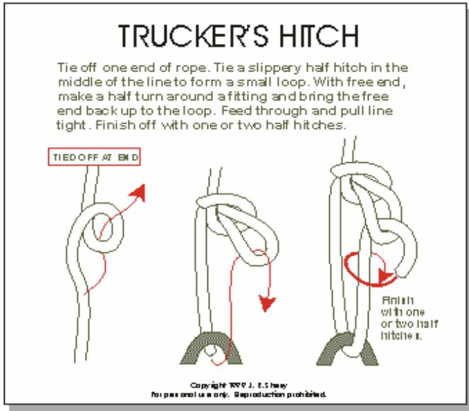
Generally, you do not want to pull the wing tie-down rope too tight (the trucker's hitch acts like a pulley and can easily put significant stress on the wing) , but you also don't want the wing to be flapping in the breeze. Simply snug down the tie-down rope, not tight, not lose (no slack).
